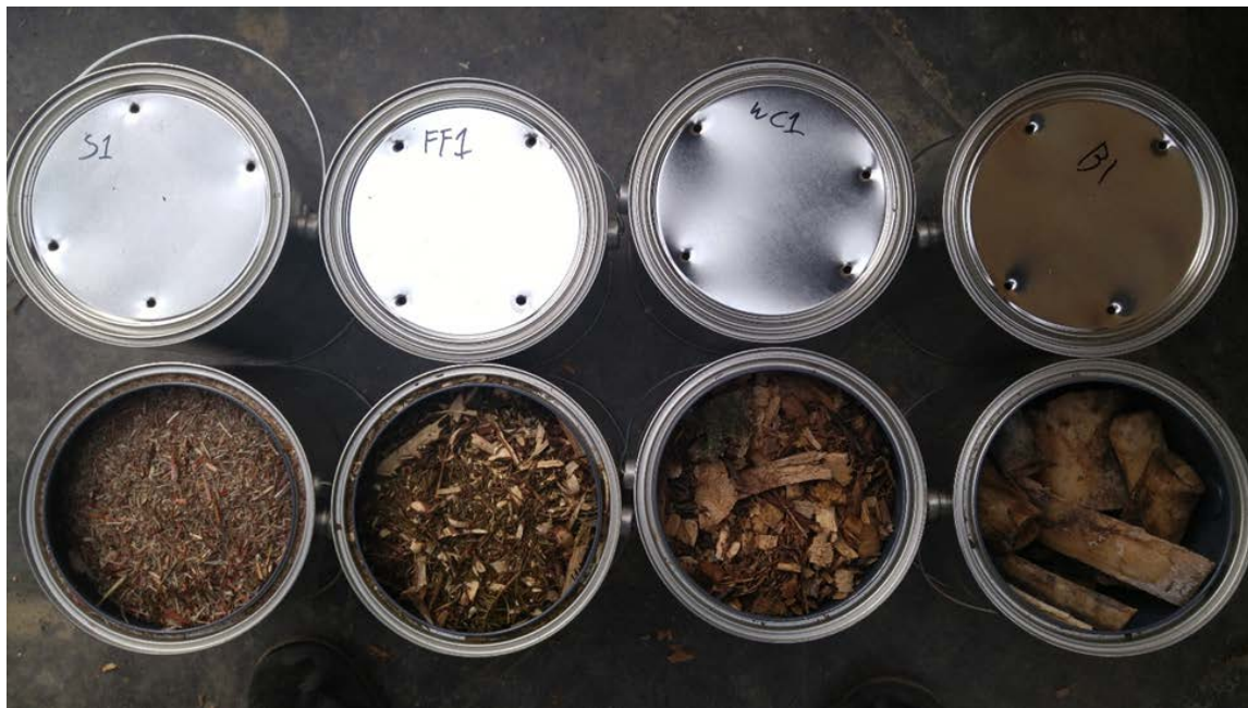
Figure 2: Biochar feedstocks. from left to right, sorghum, Fraser fir, wood chip, and bone.
