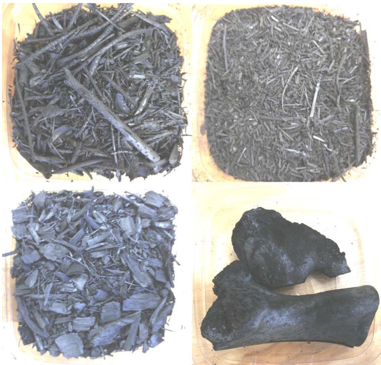
Figure 3: Pyrolyzed feedstocks, biochar before grinding. Clockwise from top left: Fraser fir, sorghum, bone, and wood chip.
